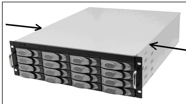
Figure A-1. Remove the Top Cover Side Screws
