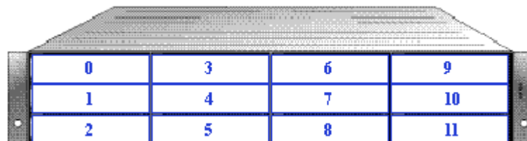
Figure 2-3. Drive Numbers on the Primary Array
