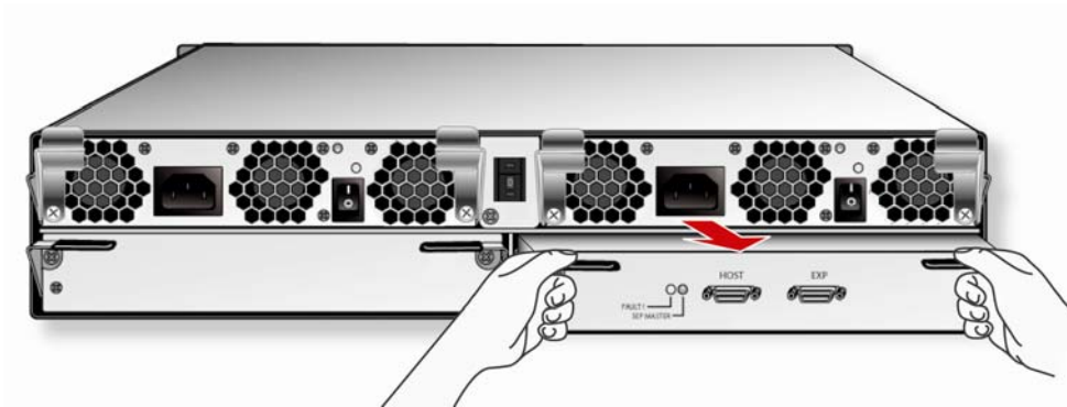
Figure A-5. Removing the I/O Module on the Expansion Array (Slot #0 shown)
